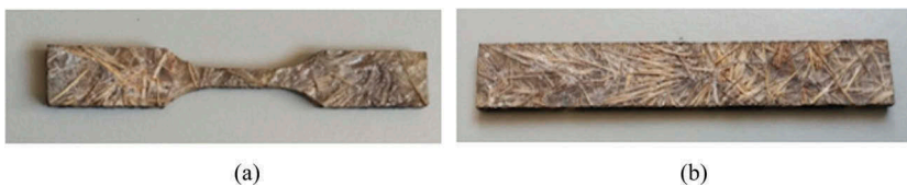
Figure 3. Specimens used for tensile test (a) and for three-point flexural test (b).
