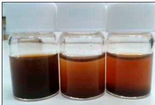
Figure 4. Colloidal stability of the magnetic cores in distilled water with extracts of R. ulmifolius flowers, T. communis shoots and C. monogyna flowers, from left to right respectively.
