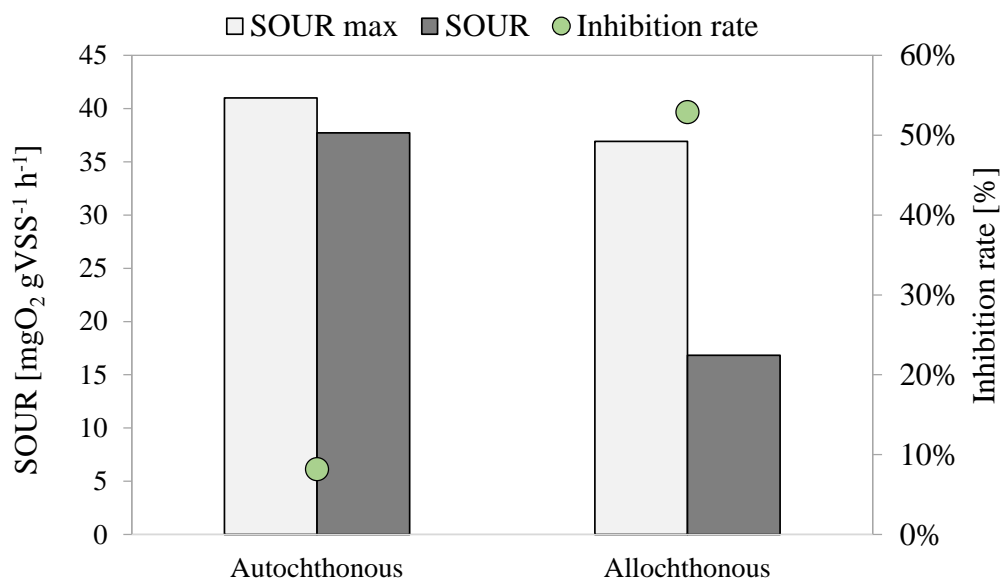
Fig. 4: Values of the SOUR and the inhibitory rates obtained during the inhibitory test performed on the autochthonous and allochthonous biomasses
