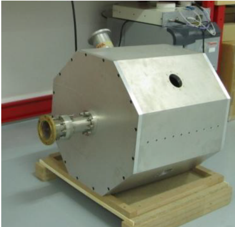
Figure 6.9: Picture of the final prototype of the RFQ fabricated in aluminum.
