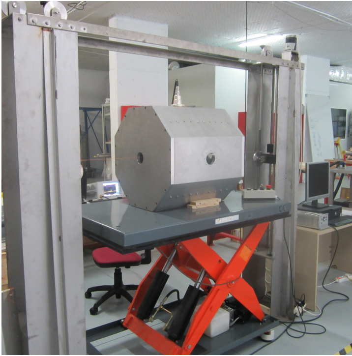
Figure 6.10: Experimental set up used for measuring the RF response of the aluminum prototype.
