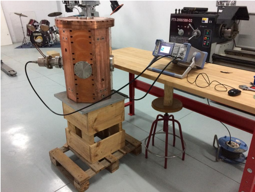
Figure 6.21: Set up for RF test of the copper prototype.
