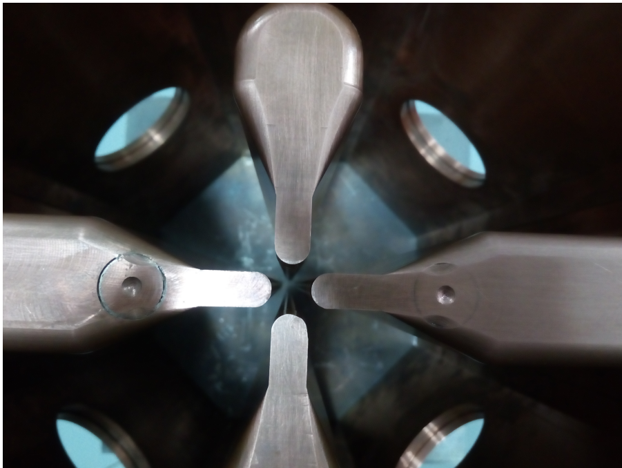
Figure 6.19: Inside view of a copper prototype of the RFQ section.
