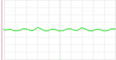
Neutral current with passive and active filter. 4 A/div. 5ms/div
