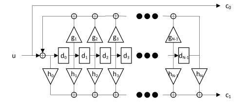
**Figure 1.** Architecture of a recursive systematic convolutional (RSC) encoder with  $R = \frac{1}{2}$ .
