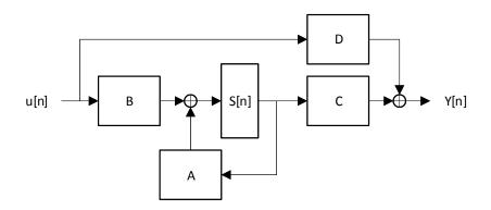
Figure 2. Block diagram of the ABCD matrices model of an RSC encoder.
