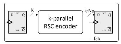
Figure 5. RSC encoder in a scenario with synchronous source and sink registers.
