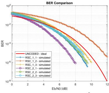
**Figure 6.** RSC encoders bit error rate  $(BER) = BER(\frac{E_b}{N_0})$  curves.
