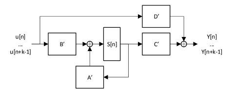
Figure 3. Block diagram of a *k*-parallel RSC encoder
