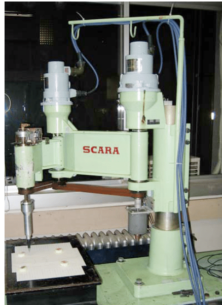
Figure 7. One of the first prototypes of SCARA robot, designed by Hiroshi Makino.
