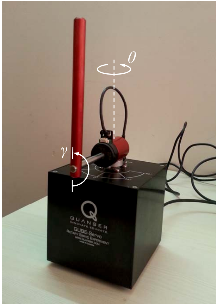
FIGURE 3.8: Rotary inverted pendulum apparatus, shown here with \theta \approx 0^\circ and \gamma \approx 180^\circ .
