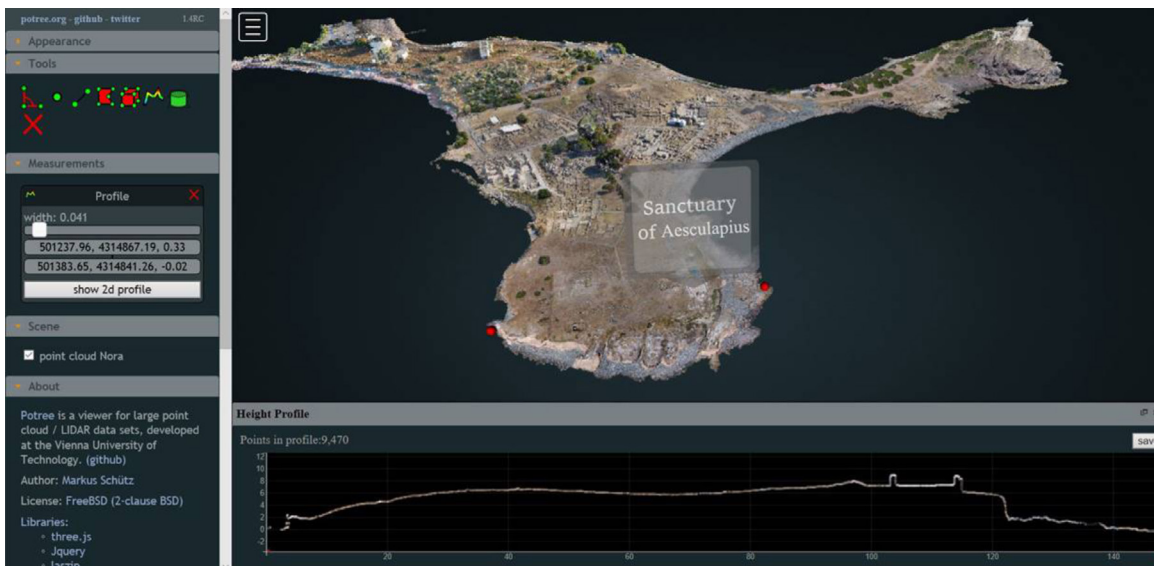
Figure 5. Potree's interface. The web renderer shows the point cloud of the site, providing a toolbox for geometrical analyses of the model. One of these tools produces the profile along a cross-section, as shown on the bottom window. Labels on the point cloud semantically inform the model.
