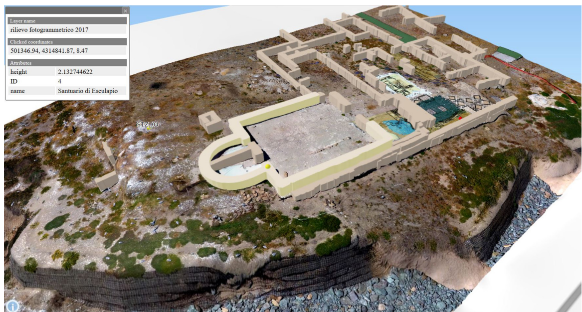
Figure 6. WebGIS page by Qgis2threejs. The plugin's output in an HTML page preserving height values and attributes for every feature.
