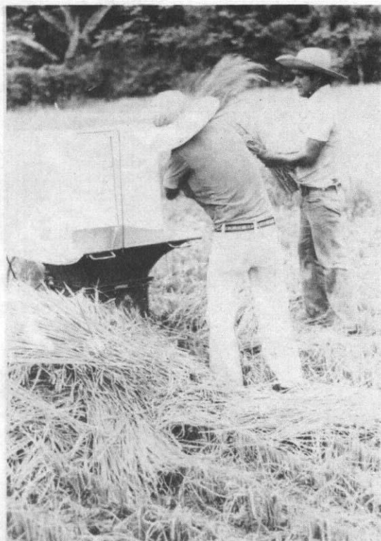
Research station trial with rice of thresher designed by CIAT, Colombia.
