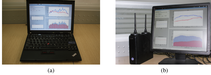
Fig. 9. Receiver setup: (a) a laptop equipped with internal Intel 5300 NIC; (b) a mini PC with external Intel 5300 NIC.
