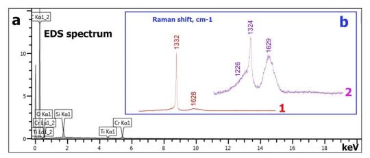
**Figure. 5.** Spectroscopic data of the general Kara impact diamond varieties: a – typical chemical composition for sugar-like diamond, energy dispersive spectrum; Raman spectra – 1 sugar-like diamond, 2 – diamond fossil
