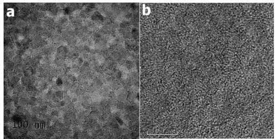
**Figure. 6.** (HR)TEM images of Kara impact diamond varieties: a – sugar-like diamond with 20-30 nm crystallites, diamond fossil with ultra-nanocrystalline structure.
