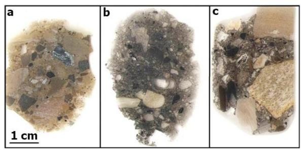
**Figure 2**. Varieties of suevites of the Kara impact crater, typical thin sections in transparent non-polarized light: a – type I suevite; b – type II suevite; c – type III suevite.
