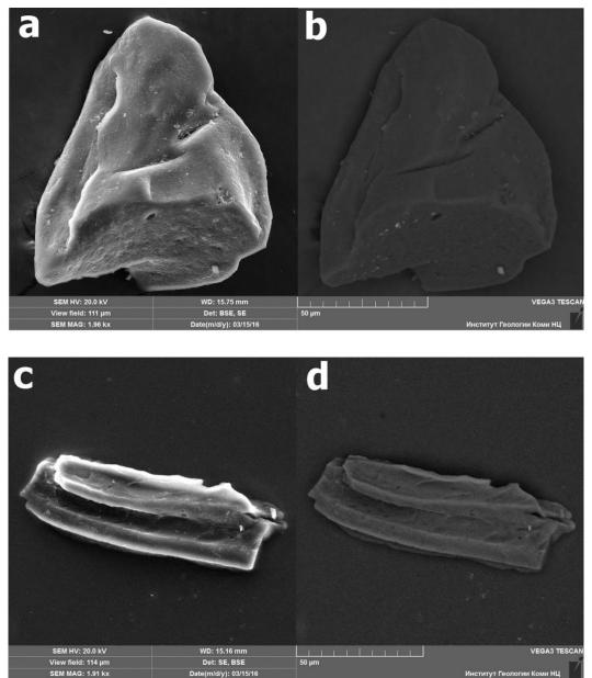
**Figure 4.** Typical diamond grains, SEM images: a, b – sugar-like diamond, c, d – diamond fossil, morphology clearly indicates the organic relict precursor. a, c – images in secondary electrons mode; b, d – in back scattered electron mode.
