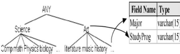
Fig. 2. The transformation of the concept tree for Major into hierarchy_major table
