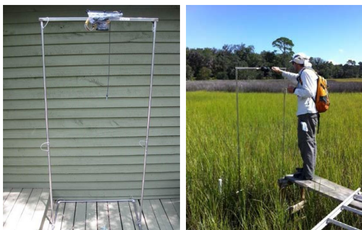
Figure 1.15. Assembled lightweight camera stand for close-to-earth remote sensing (left) and acquisition of nadir images (right). Photo credit: GTMNERR
