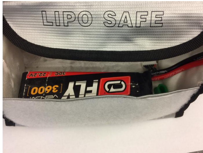
Figure 9: Proper storage of LiPo battery.
