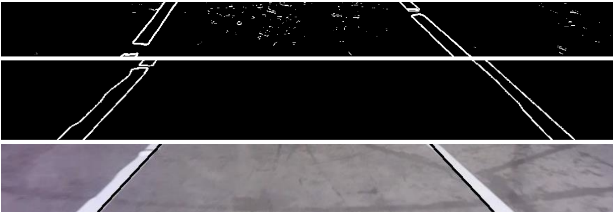
Figure 103. The first photo shows the output of the sobel filter which outputs white for any edge detected in the image. The second photo shows the result of filtering out the noise by ignoring non-white pixels. The last image shows the predicted lane lines (black) overlaying the actual lane lines (white) resulting from the output of the hough transform.
