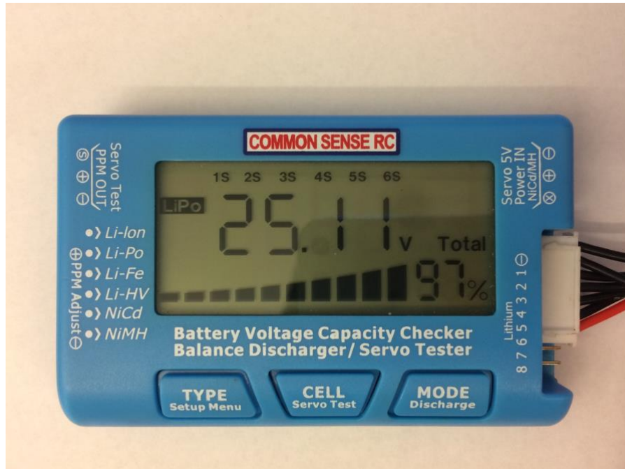
Figure 2: Checking battery cell voltages.
