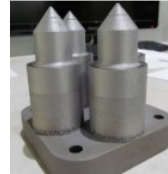
Figure 5a. Printed injection moulding inserts
