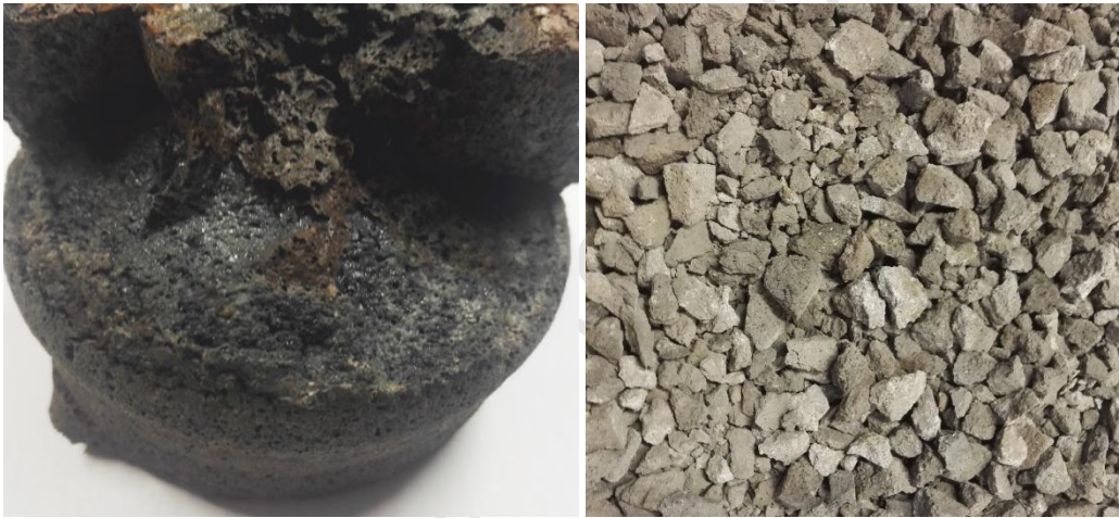
Fig. 1. Left; AOD_C after firing and removing from the crucible. Right; Fe_C after firing and crushing with hammer.
