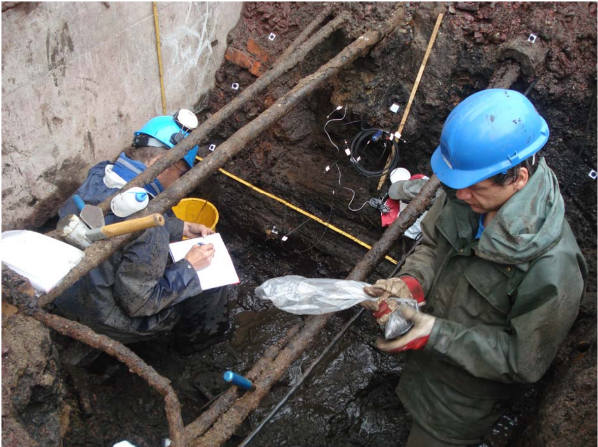
Figure 3: Field work at the excavated north eastern profile. On the left the girder is shown. The tubes that reach over the pit are electric power cables.
