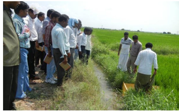
RBC flume water measurement in fields with machine transplantation at Rangareddy palem
