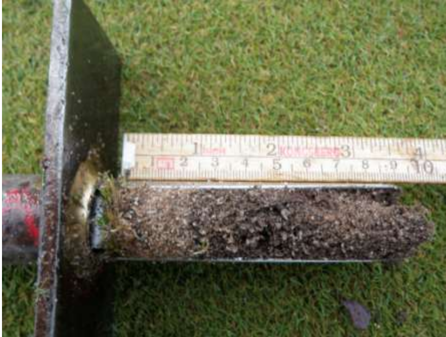
Photo 5. Measurement of thatch/mat thickness at Landvik, October 2010. Photo: Trygve S. Aamlid.
