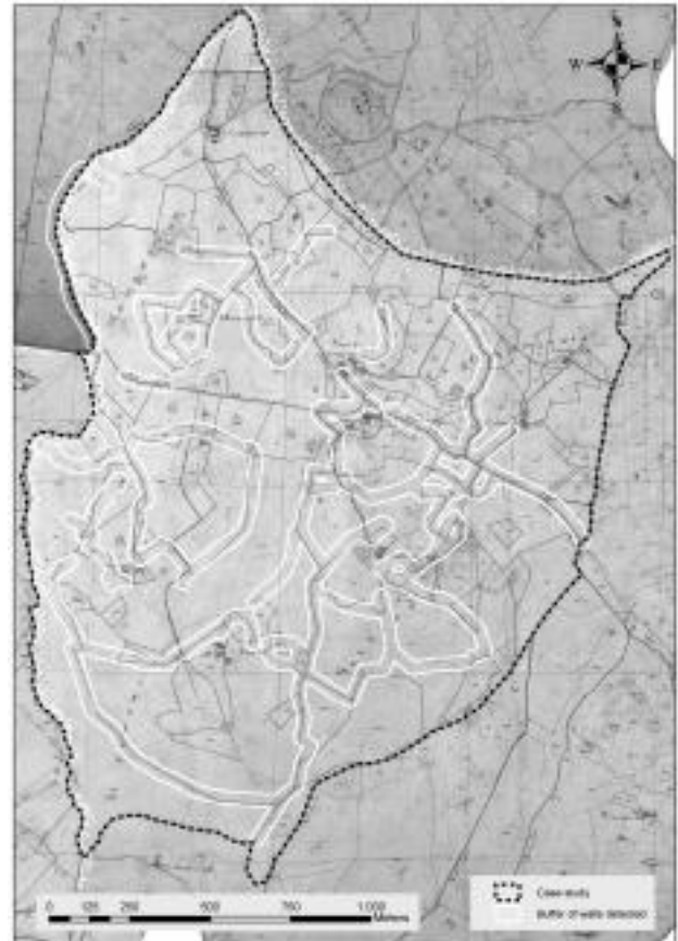
Fig. 1 - General map of the case study showing the matching between Cadastral boundary and the self-standing dry stone walls surveyed where the buffer has been set up.
