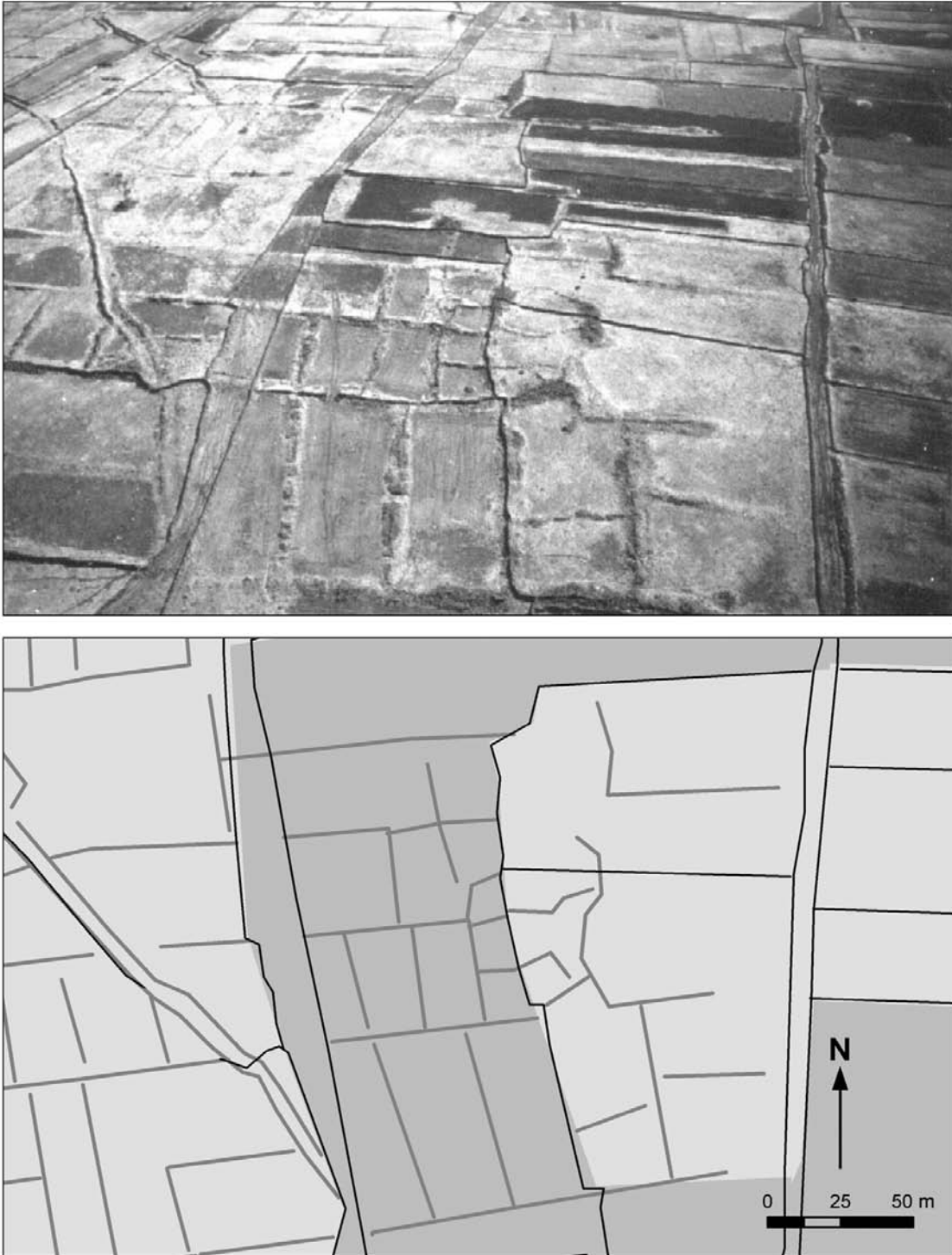
Figure 5. The same area of fields to the west of Krad Dasiniyah is shown on an aerial photograph and a Geographical Information System (GIS) coverage. Of those walls recorded using a hand-held GPS unit, the GIS coverage is able to highlight the attributes for different wall matrices. Hence, the thin black lines represent thin modern walls of one metre in height, the grey lines older wall fragments of more than one metre in width. The dark grey areas are ploughed fields, the light grey are unploughed. (Photograph: M. Abdulkarim).
