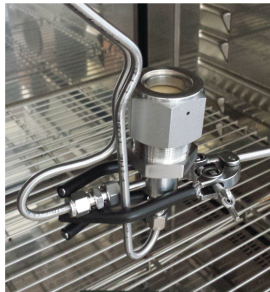
Figure 5. Prototype system for generating moisture gradient in a sample, for calibration of surface moisture sensors.
