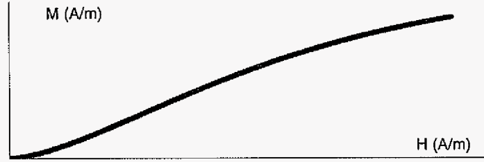
Figure 26. Phase I: the initial hysteresis loop of the Jiles-Atherton Model
