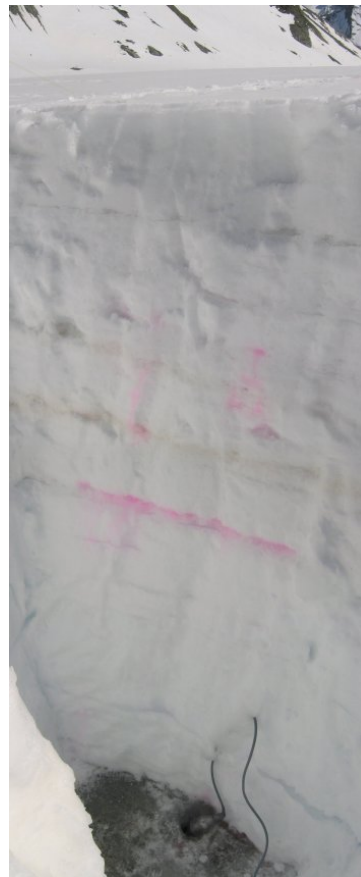
Figure 4.35: Emergence of dye from a surface injection on 8 th June along ice layers between 1.2 and 1.7 m above the glacier ice surface. Multiple individual plumes of dye emerging along the ice layer at 1.2m from ice surface have merged together to form a continuous line of pink.
