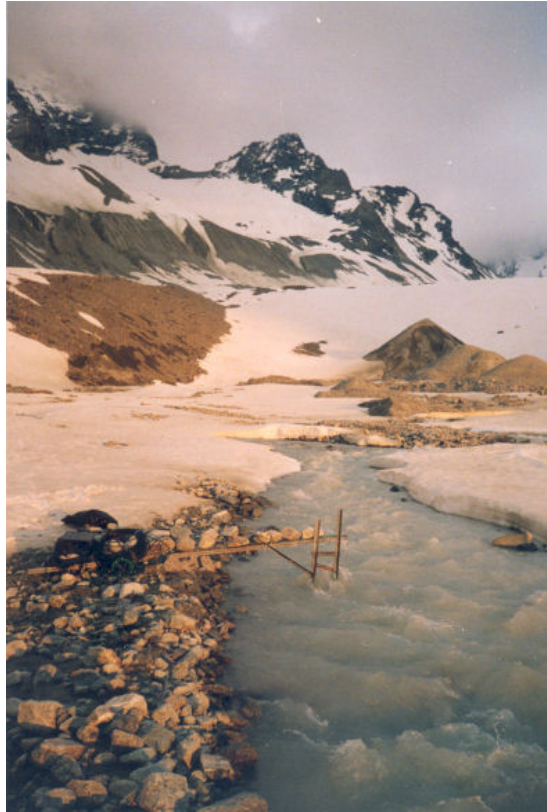
Figure 3.15: Gauging structure on the proglacial stream during the 2003 field season.
