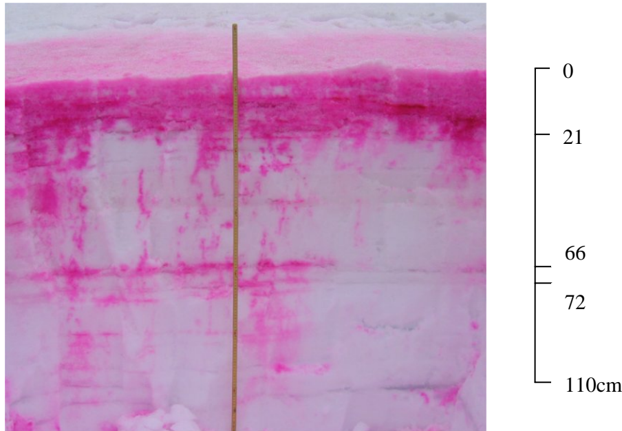
Figure 4.23: Percolation pattern at L on 16 th June 2004, 2 hours after dye injection, showing fairly even percolation through the top 21 cm of the snowpack despite the presence of two large ice layers and, beneath that, further percolation to a maximum depth of ~110 cm via multiple small flow paths. Ice layers at 66 and 72 cm depth have retained some dye but allowed some to pass.
