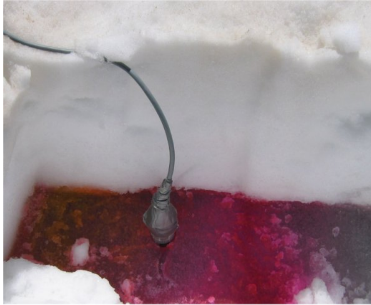
Figure 3.7: Fluorometer installation beside the upglacier wall of a snowpit to detect dye arriving in the basal saturated layer. The glacier ice surface slopes downslope towards the camera; dye was injected upglacier and can be seen arriving in the saturated layer behind the fluorometer. The fluorometer is sitting in a shallow borehole to ensure that water flows past its sensors.
