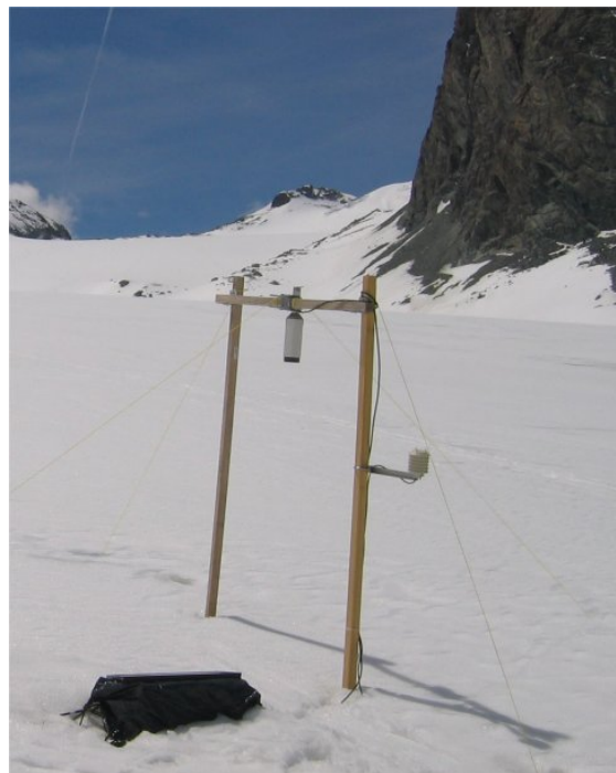
Figure 3.13: Ultrasonic depth gauge (UDG) mounted on 'H' frame and anchored using guy ropes to decrease instrument movement in windy conditions and therefore increase measurement stability. The thermistor used to correct UDG distance measurements for air temperature is mounted inside the radiation shield on the right hand post.
