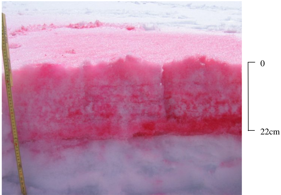
Figure 4.20: Percolation pattern at L on 29 th May 2004, 45 minutes after dye injection. Dye has percolated to a major ice layer 22 cm from the surface and is retained above it. Dye percolation has taken place via multiple small (~1 to 2 cm diameter) flow fingers, giving the dyed area a ‘marbled’ appearance.
