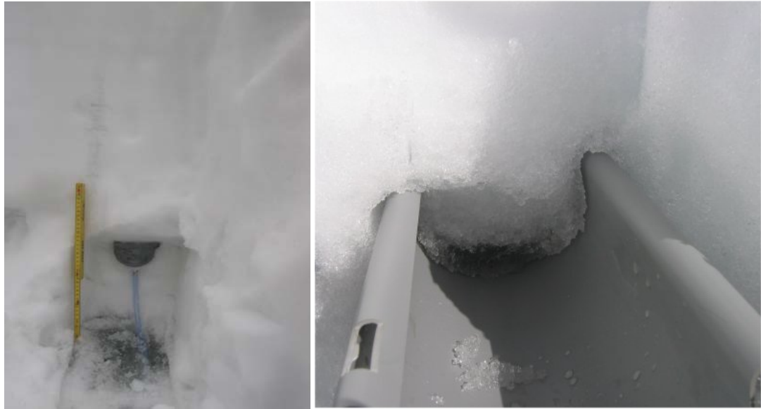
Figure 3.11: Drainpipe lysimeter installation: a) lysimeter installed in pit wall; b) water saturating the snow in the lysimeter immediately after installation into the snowpack.
