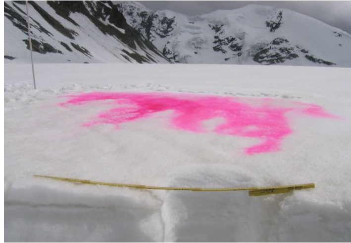
Figure 4.24: Retention of dye above a near-surface ice layer on 21 st June 2004 (~1.5hrs after injection), believed to be triggered by refreezing of the ice layer in cold weather. Photograph looks in the upglacier direction. Ruler in foreground is 1m in length.
