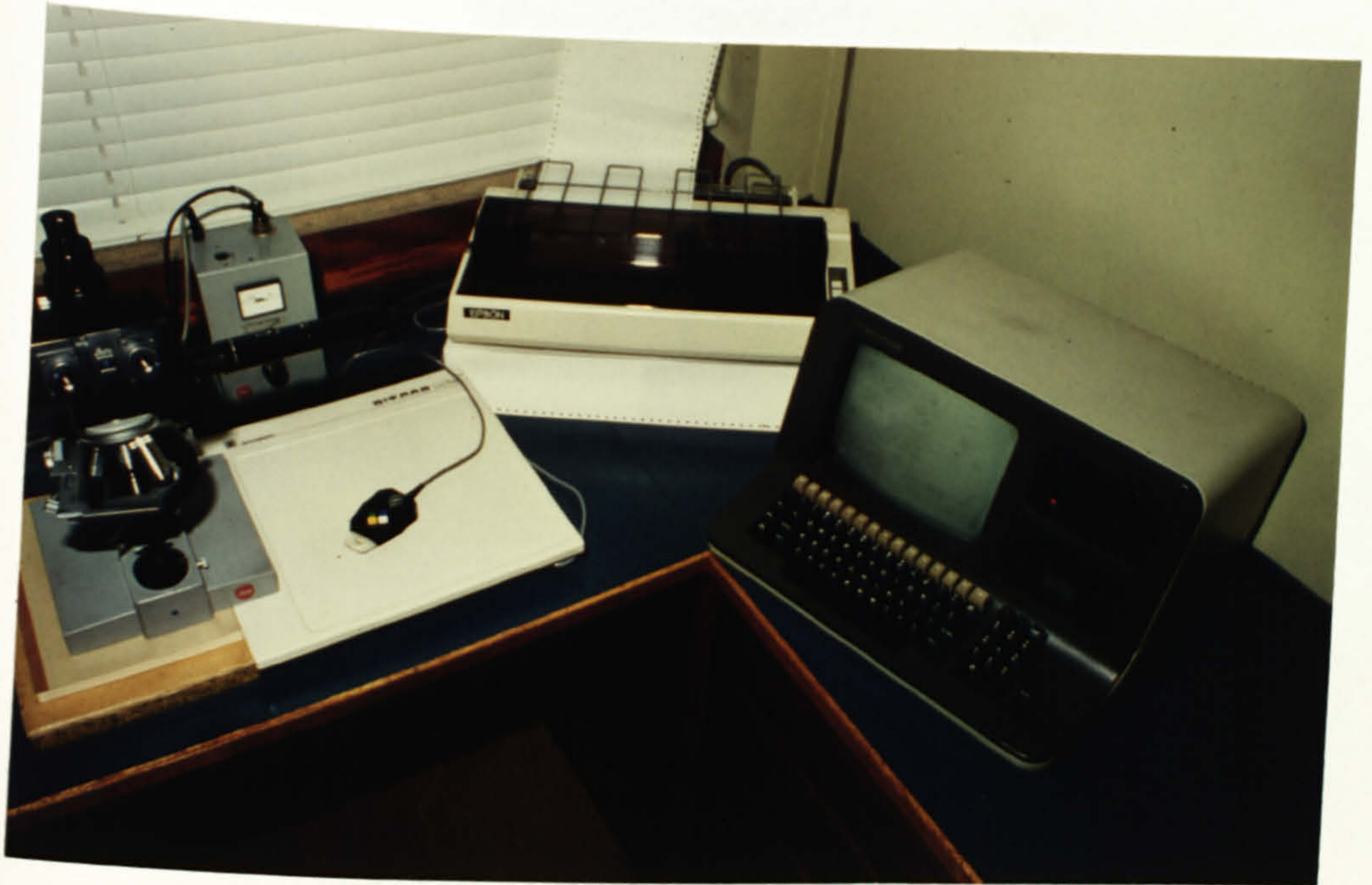
FIGURE 2.5 The features of the computerised planimetry system used for the compartment analysis of the hamster cheek pouch epithelium.
