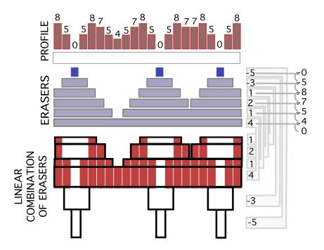
Figure 5.1: Combination of SEs that match a lexical neighbourhood profile. A combination of six SEs with the appropriate weights can reproduce the profile shown in the upper part of the graph. The combination W = -5E(t, 0) - 3E(t, 1) + E(t, 2) + 2E(t, 3) + E(t, 4) + 4E(t, 5) would scale the different positions around t in 0, 5, 8, 7, 5 and 4 according to the distance to the central term.
