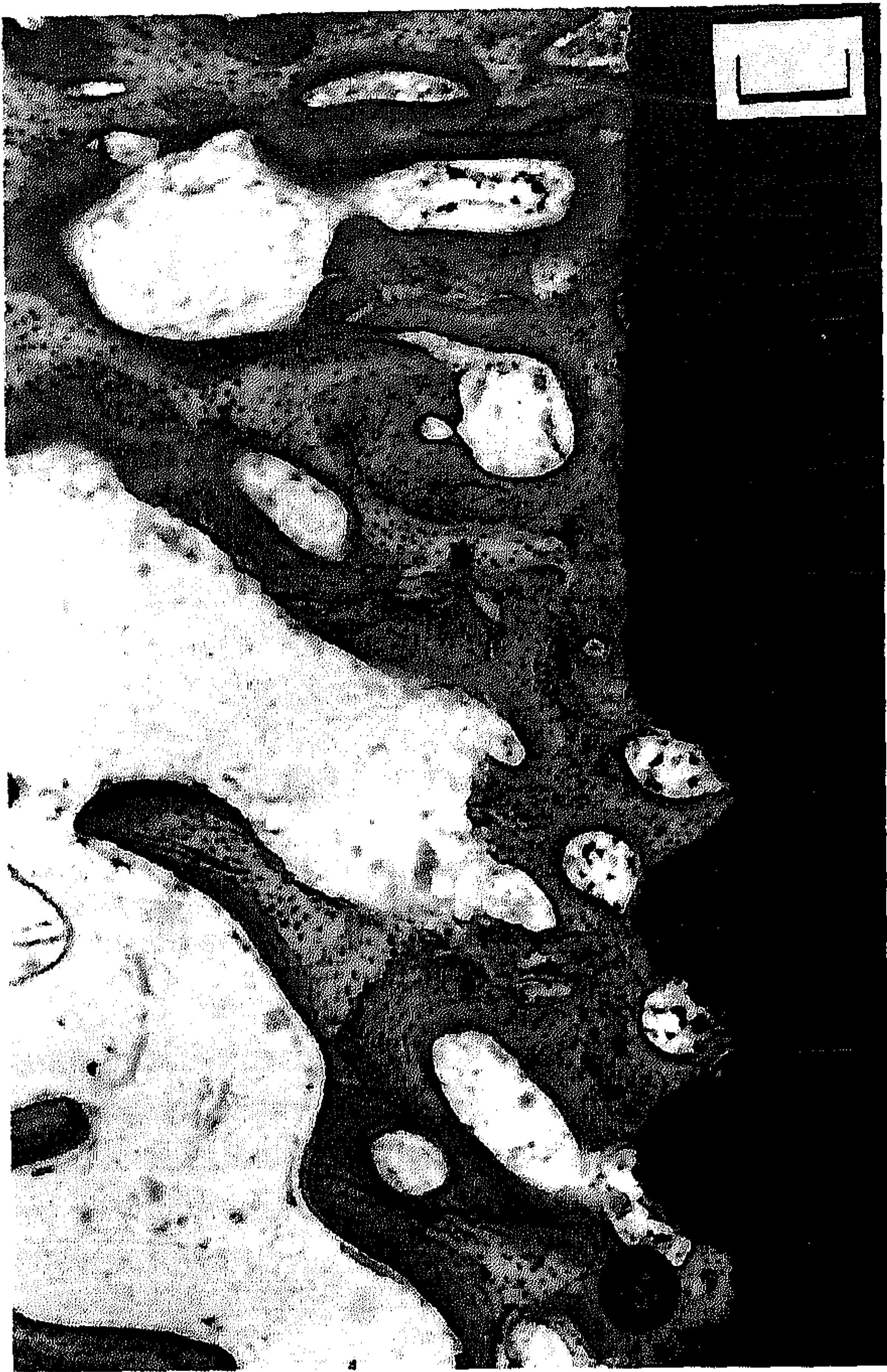
Figure 7. Histologic section of an FA/HA-PS-coated implant after 3 months of implantation. In the screw threads the coating has partially disappeared. The trabecular structure of the bone around the implant can clearly be recognized. Bar = 300 \mu\text{m} .
