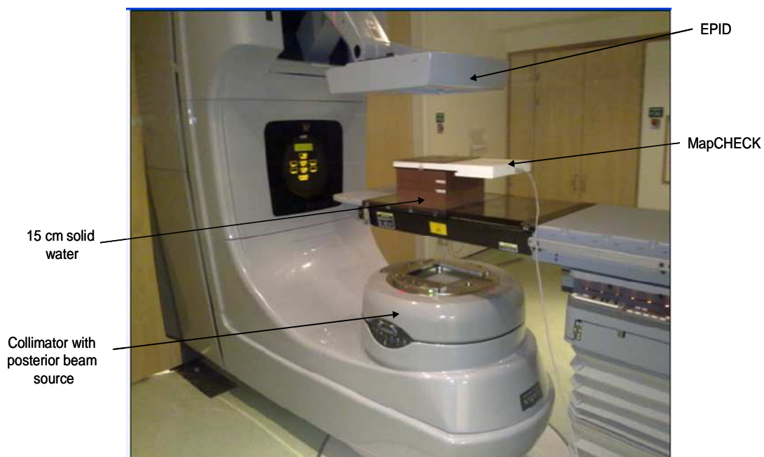
Figure 3- 12: The setup used for the simultaneous MapCHECK measurement and EPID image acquisitions.
