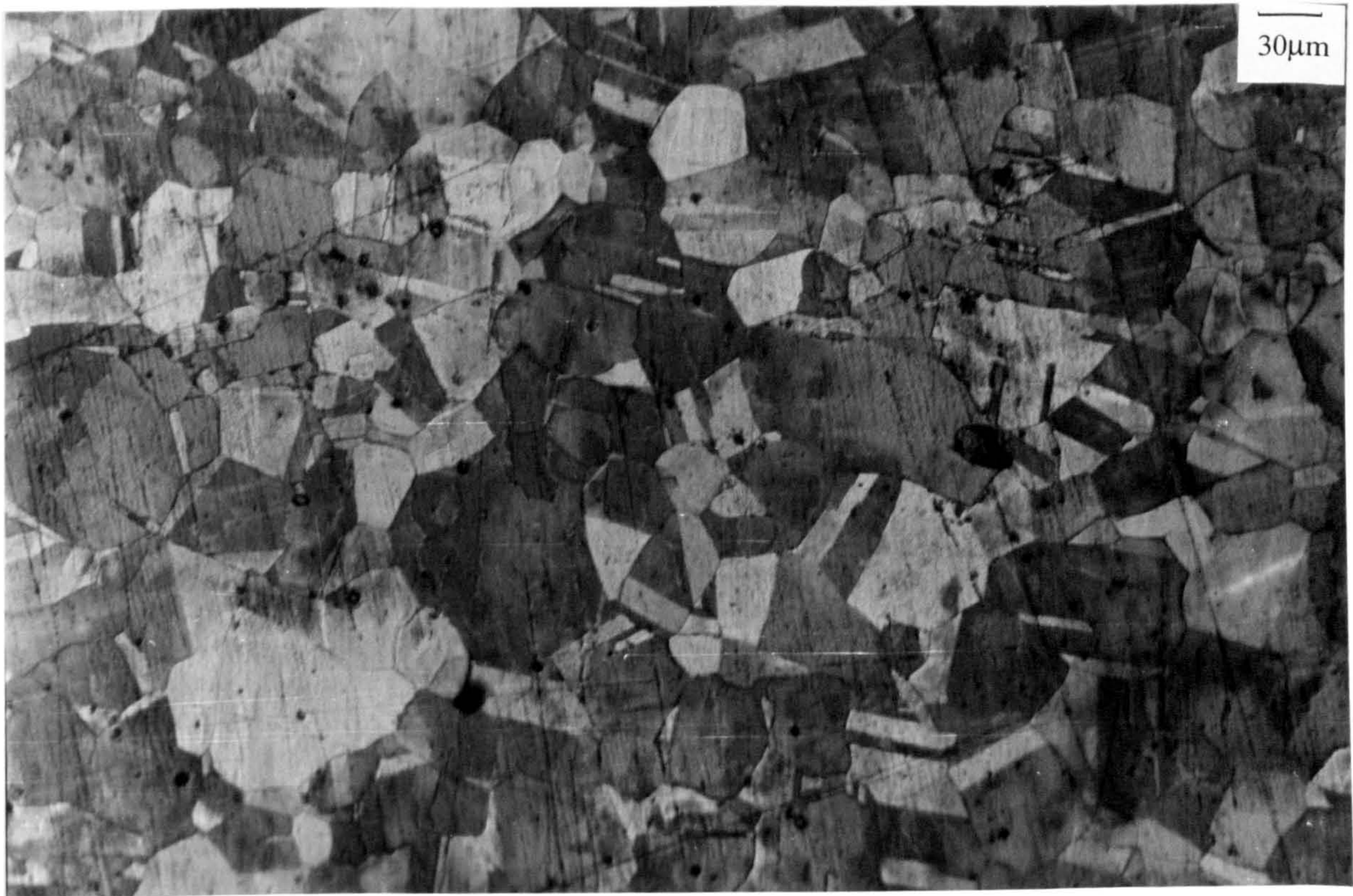
Figure 7.12. Cu-10%Ni, V=17\text{m/s} , 8 hours, \phi=45^\circ , T.W.L. The etched structure evident on the whole surface.
