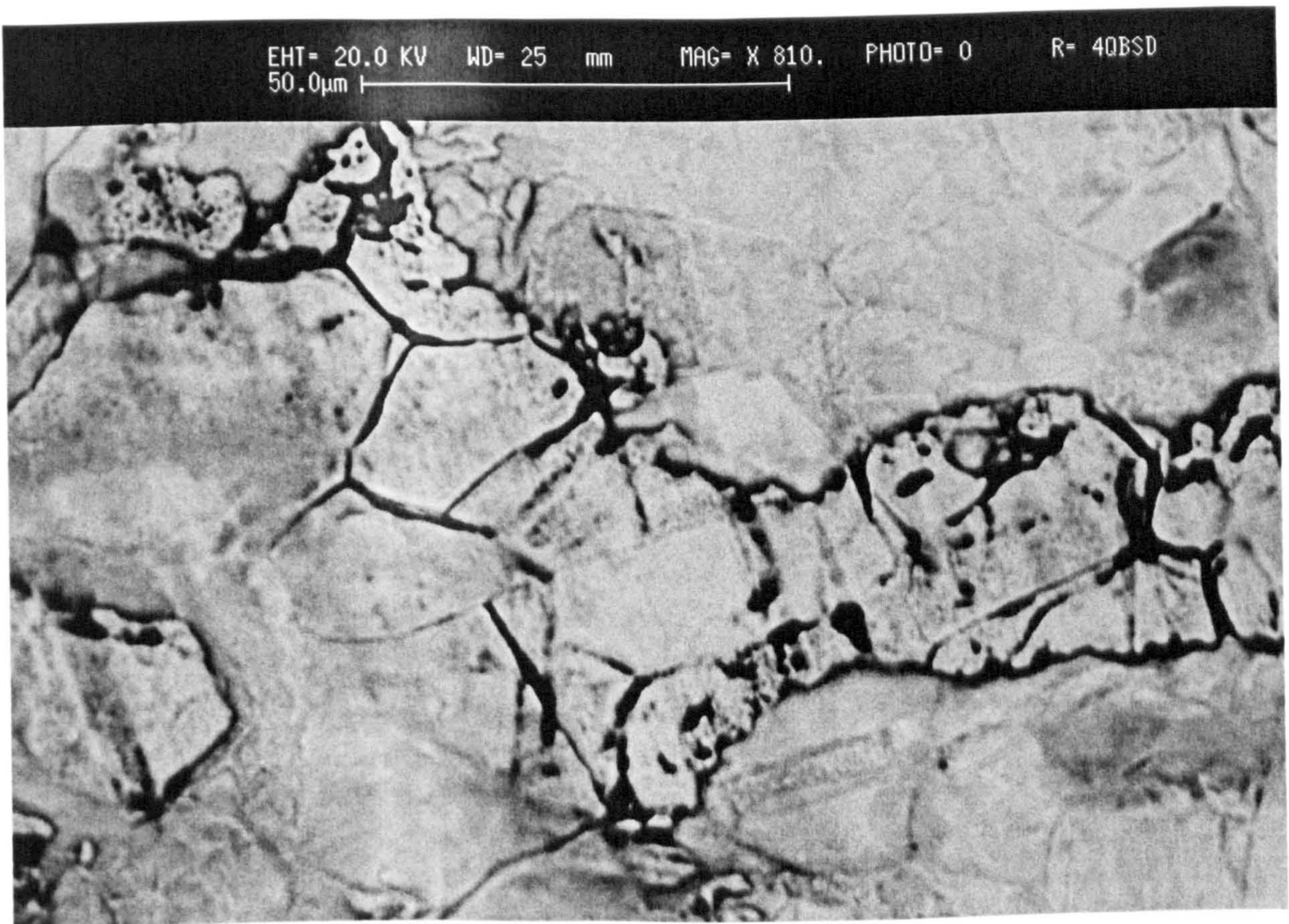
Figure 7.17. Cu-10%Ni, V=17m/s, 48 hours, T=35°C, T.W.L. The variations in film structure and thickness.
