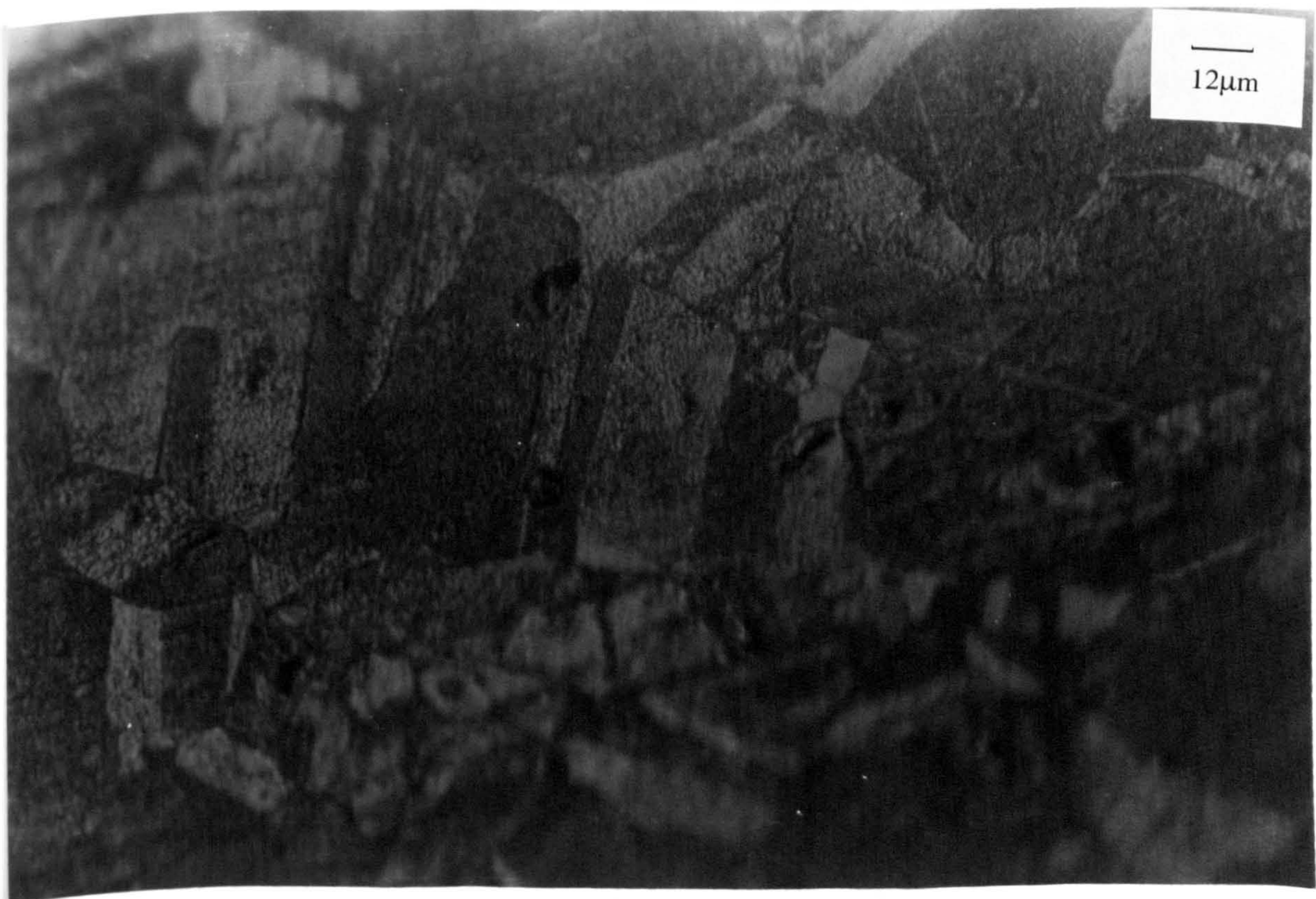
Figure 8.14. Cu-10%Ni, Concentric, V=17m/s, 72hours, T=35°C, T.W.L. A black film covered the entire surface with the etched structure underneath the film still visible.
