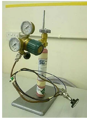
Fig 2.3: 200 psi CO 2 regulator with compressed ^{13}\text{CO}_2 cylinder
