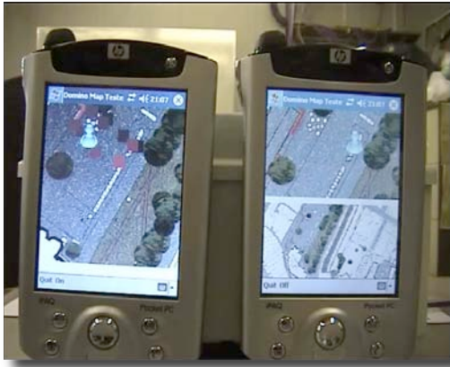
Figure 37: Domino map layer test application. One device has a map viewer with two layers: pollution and GPS. Another device has two viewers and at present only the GPS layer.
