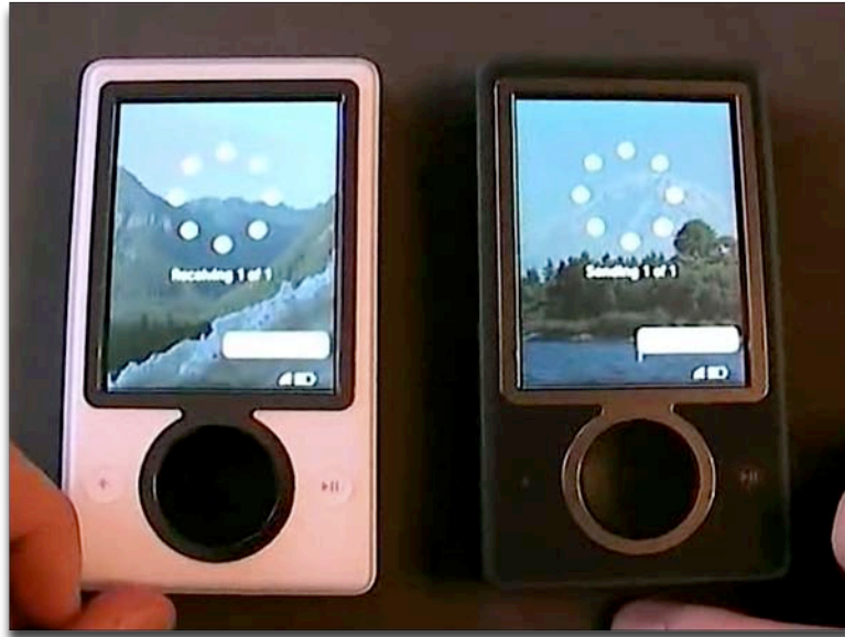
Figure 20: The Zune MP3 player exploits ad hoc WiFi connection to exchange music files.
