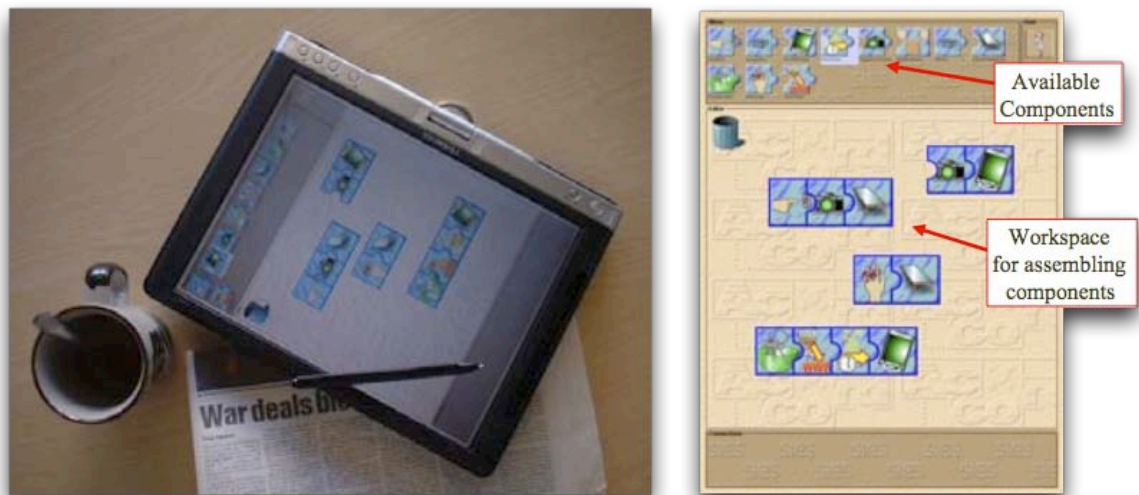
Figure 31: The Jigsaw user interface for connecting jigsaw pieces representing sensors, devices and services in ubiquitous domestic environments.
