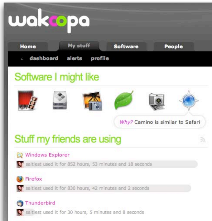
Figure 30: Wakoopa.com uses tracking software to log the use of applications, then submits this information to a web site to give recommendations for other applications based on comparisons with other users.
