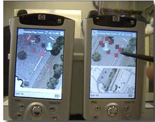
Figure 38: The pollution layer has been transferred from the PDA on the left to the PDA on the right, and is displaying in the map viewer containing the GPS layer, which it has been known to be used with.
