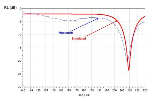
Figure 5 - 14 : Simulated and measured return loss of elevated bow-tie antenna.
