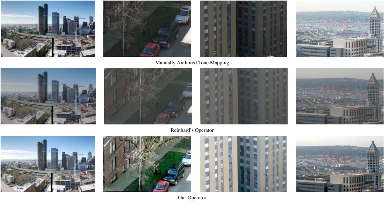
Figure 11: Different Tone Mappings. The manual tone mapping produces a great result for overviews of the full image, and respects the artistic tonal decisions of the photographer. However, when zooming into dark or bright spot of the photo one might want to enhance some details there. With Reinhard’s global operator the resulting images often look a bit washed out and also the colors seem to shift a bit. In all three case, our operator produces a good result at interactive rates.
