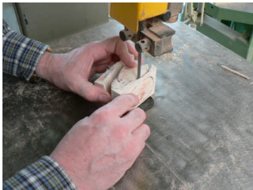
Fig. 3.35 'Carving body with cutting-saw'
