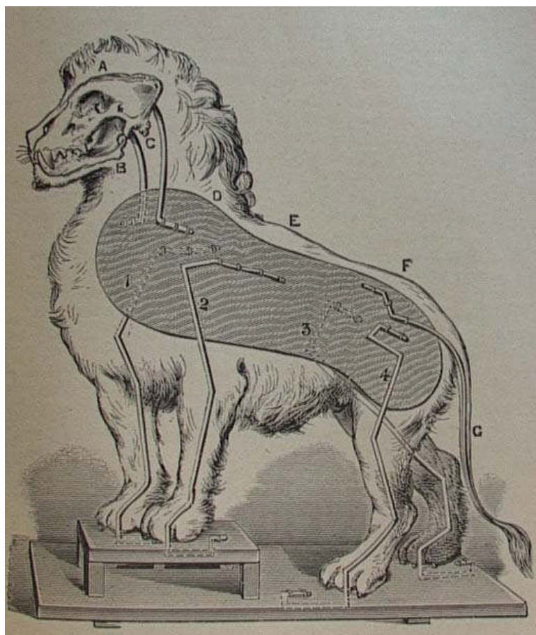
Fig. 3.43 'Lion mounted from the "flat" Showing position of 'body board' and leg irons, &c, but without false ribs' (Browne 1876: 169)
