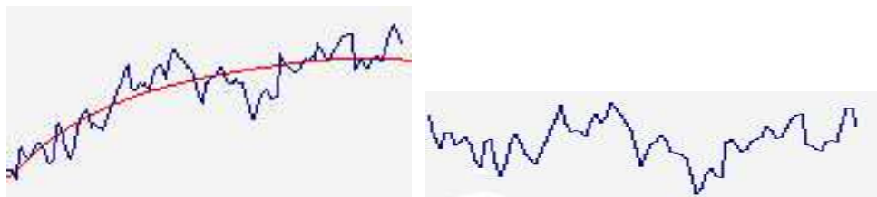
Figure 6.14 Demonstrating the removal of baseline drift from an individual waveform using the spline fitting technique. The mfERG waveform affected by drift (left) is shown in blue while the 2 nd order spline is shown in red. It can be seen from the waveform on the right that the drift has been successfully removed.
