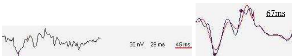
Figure 6.27 Example 4: the location of P1 as stated by the expert (left) and the spline after filtering the response (right). In this instance there was a 22ms discrepancy between the spline and the expert when analysing this noisy mfERG response.
