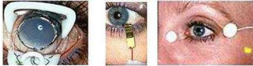
Figure 2.7 Different types of electrode used for ERG recordings. From left to right: contact lens; lid hook; and fibre electrode (adapted from www.webvision.com ).
