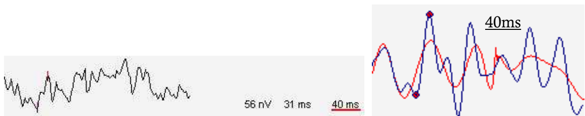
Figure 6.26 Example 3: the location of P1 as stated by the expert (left), and the spline after filtering the response. The expert and spline both identified a P1 latency of 40ms. Prior to the removal of the baseline drift and filtering there was a discrepancy of 27ms between the expert and the spline.
