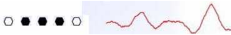
Figure 4.36 Demonstrating a small portion of an m-sequence (left) and the corresponding response (right). On the left, 5 steps of an m-sequence are illustrated, with white representing the on state (1) and black being the off state (0). The trace on the right demonstrates the response evoked from this short part of the m-sequence.
