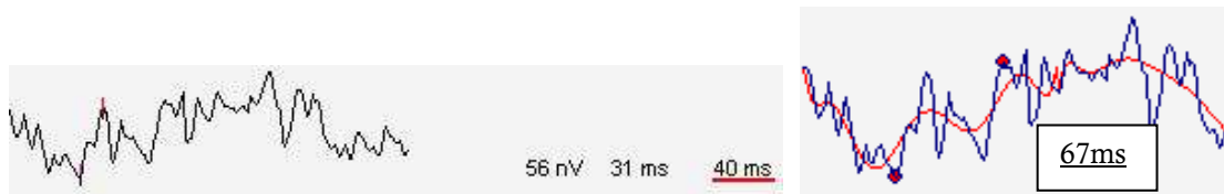
Figure 6.10 Example 3: the location of P1 as stated by the expert (left) and the spline (right). There was a 27ms discrepancy between the spline and the expert when analysing this noisy mfERG response.
