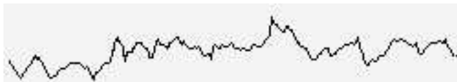
Figure 6.1 A waveform recovered by cross correlating the raw data against an unused (dead) sequence. It comprises only noise.
