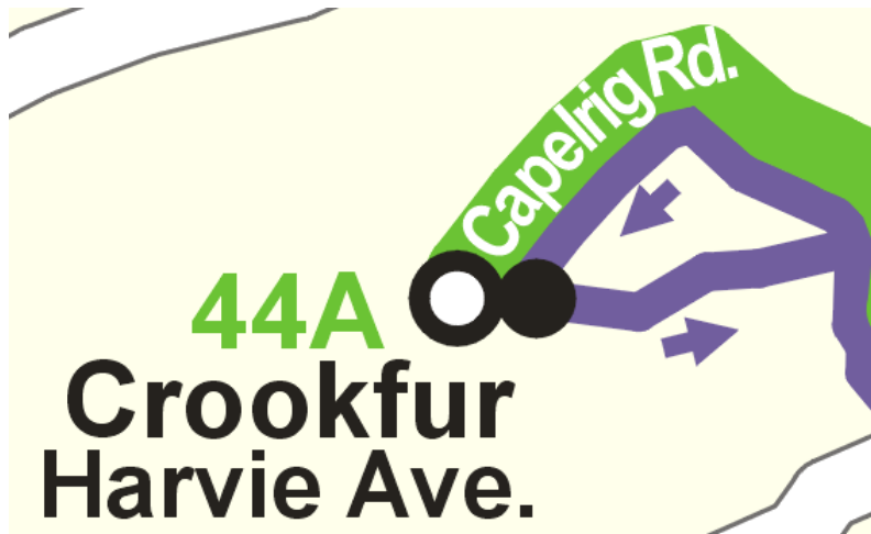
Figure 4.7: Extract of a SSBM showing the different symbols used for the termini and standard bus stops, and how the two are compatible.
