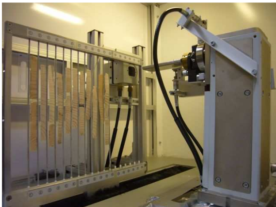
Figure 2-3. Wood samples mounted on needles on the ITRAX sample rack. The rack will move forward to bring each needle in turn in front of the x-ray beam. To scan each sample the rack lifts up step by step as defined by the step size.
