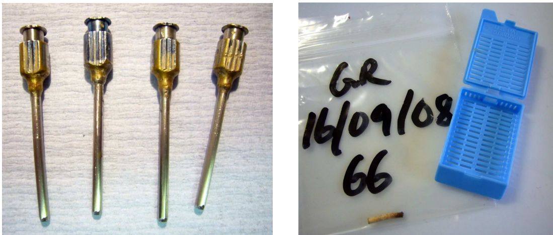
Figure 4-6. Modified medical needles used to take the microcore samples (left). A microcore and a biocassette used in the paraffin impregnation (right).
