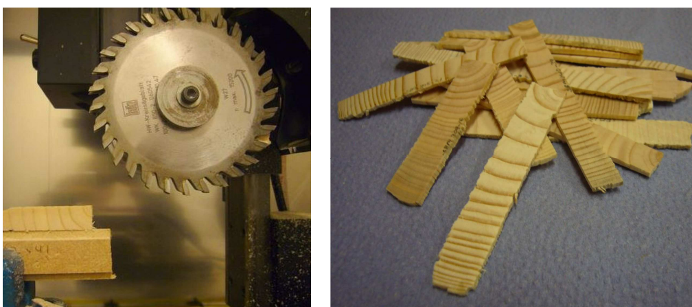
Figure 2-2. Left: a milled increment core sample on a purpose made sample holder. Right: Sample strips ready for analysis on the ITRAX X-ray densitometer.
