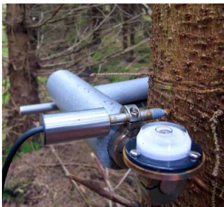
Figure 4-2. Point dendrometer on a tree at the Griffin site, Aberfeldy, Scotland.
