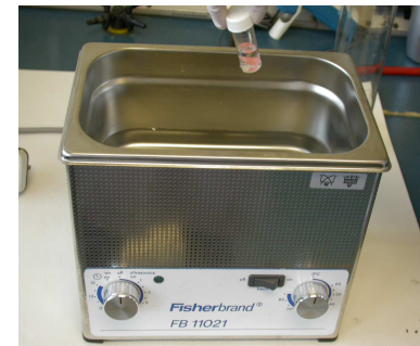
Transferred to 2ml PBS in Bijoux's tube and sonicated for 5 minutes
