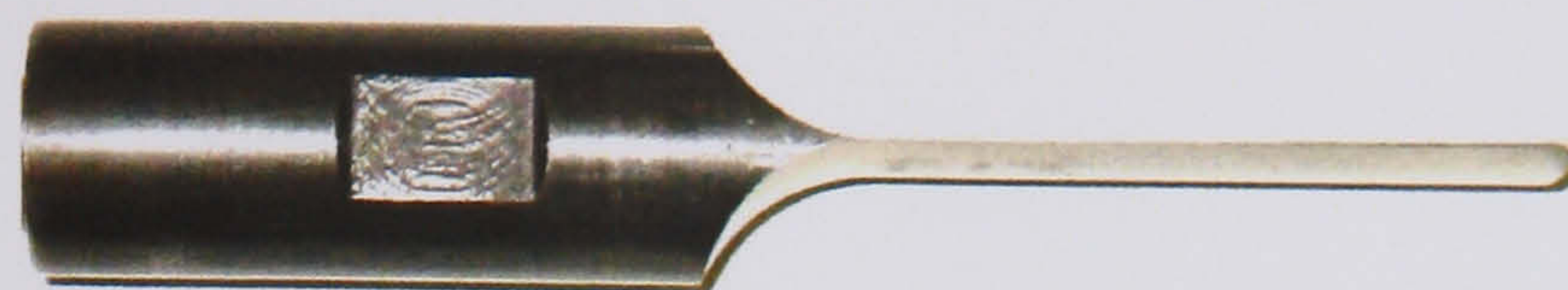
Figure 4.2: Half-wavelength 35 kHz cutting blade with vibration amplitude gain 6.
