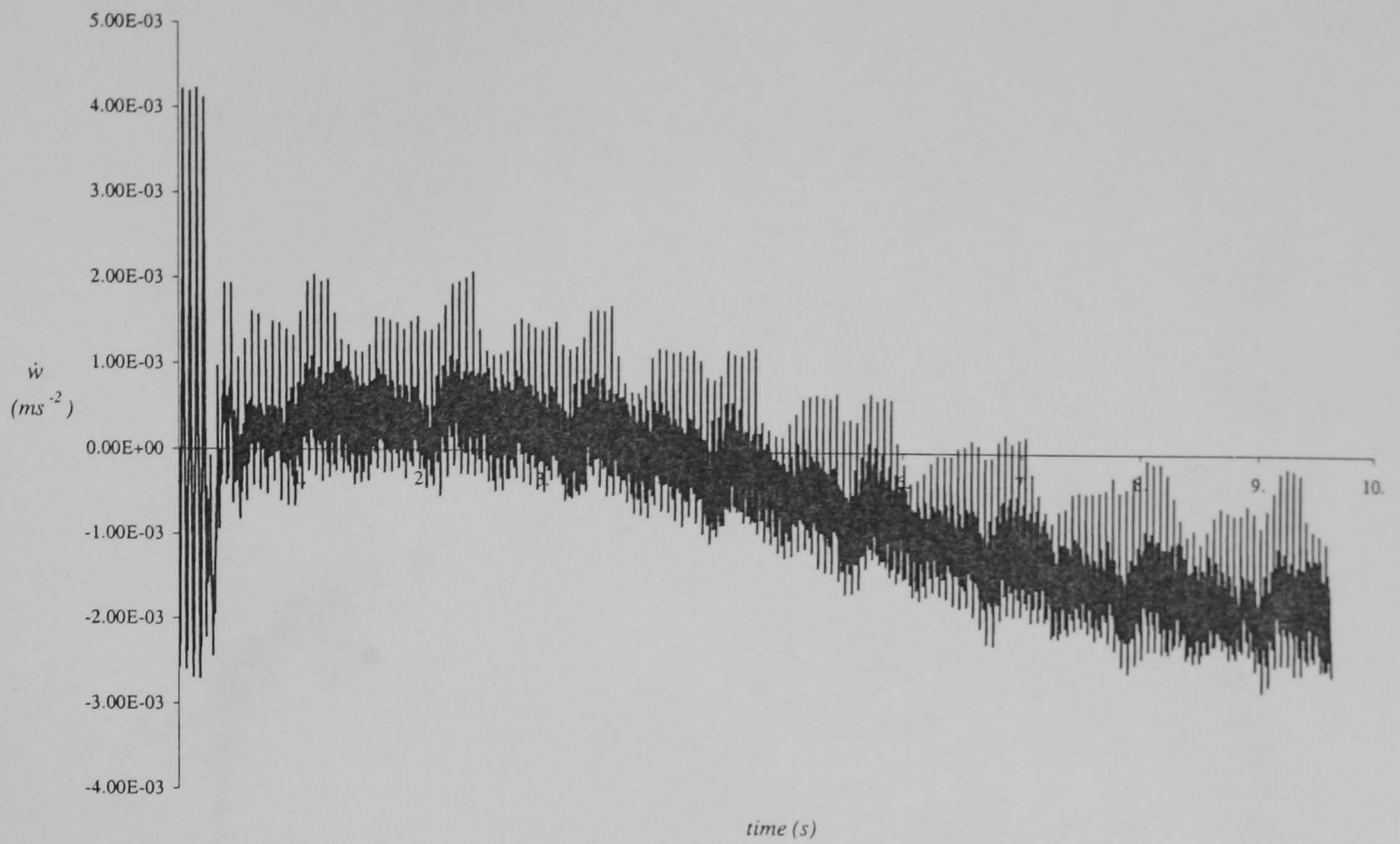
Figure (6.3) : Time History Illustrating the Performance of the Optimal HHC algorithm in attenuating still-air vibration at 20knots.
