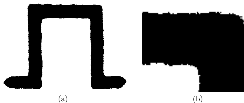
Figure 3.12: (a) Image of the mask file used in the modified simulation. A close-up of one of the corners is given in (b) where the detailed edge structure is revealed.
