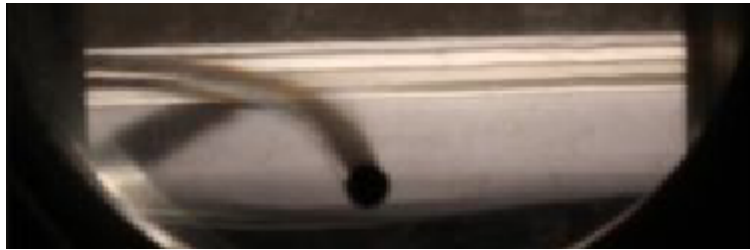
Figure 8.2: Experimental test of the predication straight line perpendicular to a ray-flipping sheet, when viewed through the sheet, appears bent into a hyperbola. The photo shows a straight metal bar that is approximately perpendicular to the ray-flipping sheet, seen through a confocal cylindrical-lenslet array, orientated such that it inverts the horizontal light-ray-direction component. The end of the bar (small back disk) touches the ray-flipping sheet.
