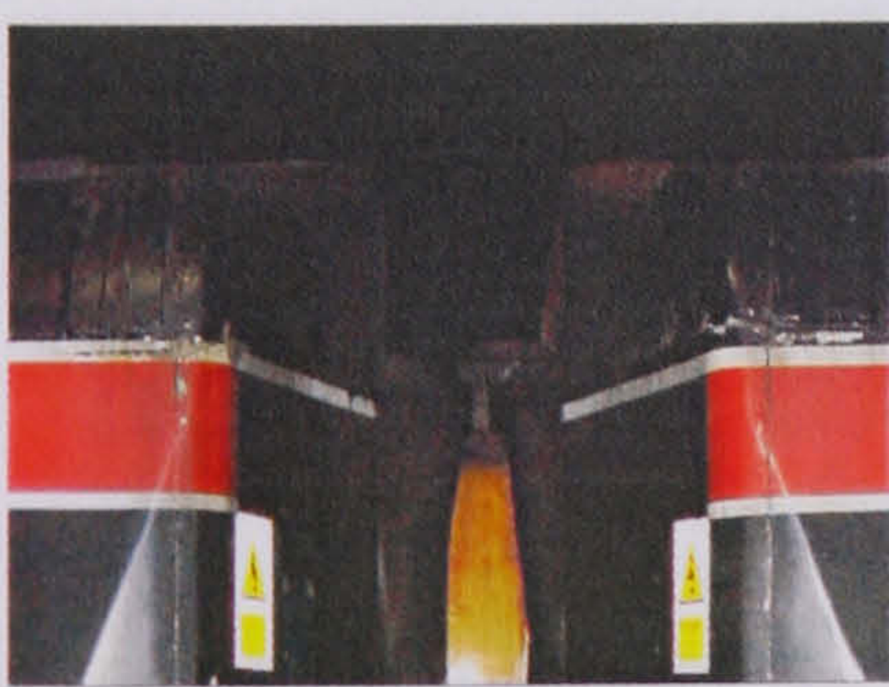
a. Train gap approximating a clean cavity with L/D = 1.0 .
