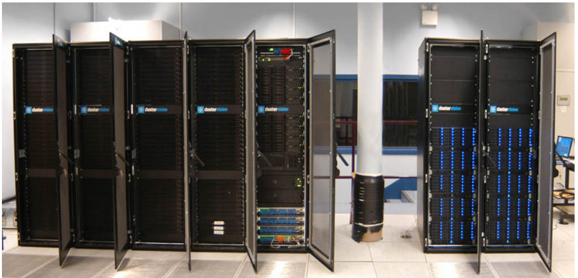
Figure 3.4 – Glasgow hosts a grid computing site dedicated to promoting grid computing within the University and supporting the wider ScotGRID project. The Glasgow ScotGRID Cluster Worker Nodes are shown above.
