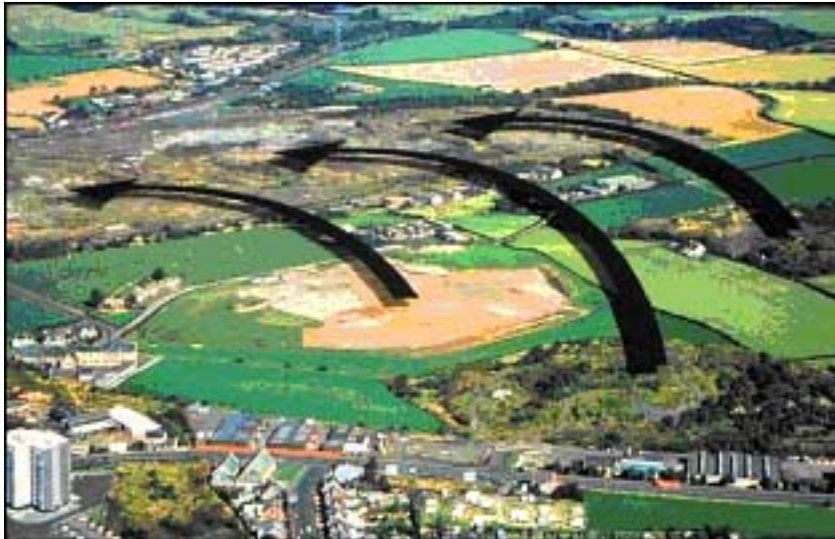
Figure 2.3 Capping Material Relocated at Hallside
