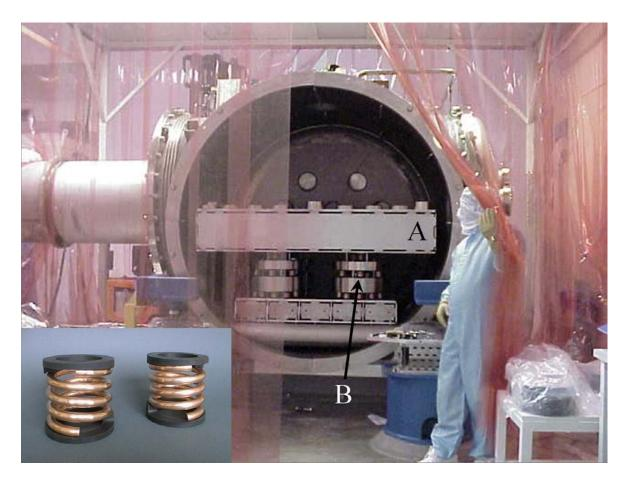
Figure 5.28: An open HAM chamber reveals the optical table (A) supported by mass spring stacks (B). Inset: Springs in more detail.
