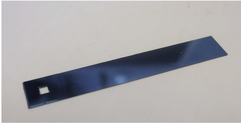
Figure 6.16: A pair of 100\mu\text{m} and 50\mu\text{m} cantilevers bonded together to form a single structure of thickness 150\mu\text{m} .
