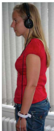
Figure 4-17: Computer-Controlled wristband with four embedded vibrotactile actuators plus headphones.
