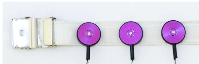
Figure 5-3: Belt lined with velcro used in experiment with 3 C2 Tactors attached.
