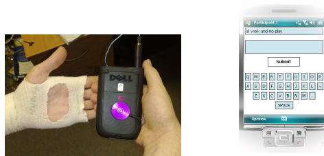
Figure 6-20: Experiment set-up with PDA, C2 Tactor, bandage securing the SHAKE to hand and text entry GUI screenshot.
