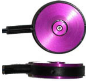
Figure 2-2: Engineering Acoustics Inc (EAI) C2 vibrotactile actuator.
