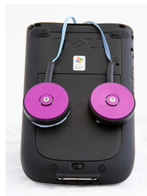
Figure 6-10: The Dell Axim PDA with 2 C2 actuators on the back.
