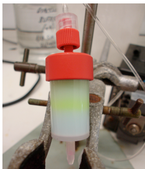
Figure 4.5: Elution of green coloured GFP-His 8 from the second affinity column.
